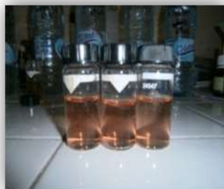
Photo 7 : Staining samples containing chlorides
